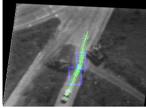
Figure 3: Trajectory of the car and the locations where it stopped (in blue).
