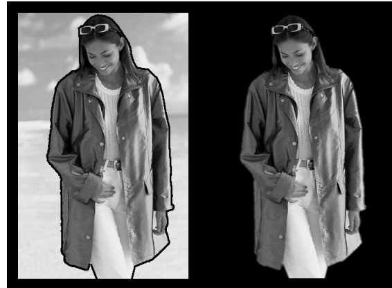
Figure 6: Screenshot from the implementation. On the left side the black segmentation path is shown. The right side shows the image with the background removed.
