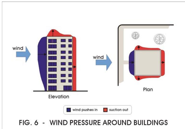
The indoor air pressure of a building may increase or decrease with wind speed depending on the number and location of openings in the envelope. Generally, if the openings are uniformly distributed on all sides of the building, the resultant indoor pressure is slightly lower than the ambient barometric pressure. The result is a slightly increased pressure difference at the windward side and a slight decreased pressure difference on all other sides, including the roof.
