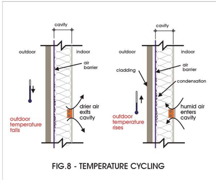
FIG.8 - TEMPERATURE CYCLING
