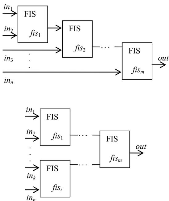
Fig.3 Types of FIS hierarchical structure
