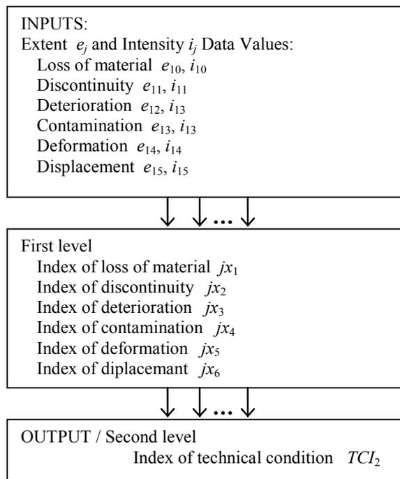
Fig.6 Fuzzy diagnostic model for evaluation of bridge substructure defects
