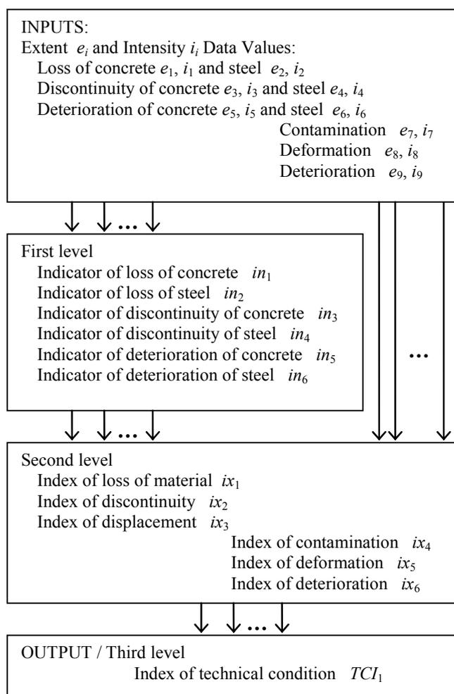
Fig.4 Fuzzy diagnostic model for evaluation of bridge superstructure defects
