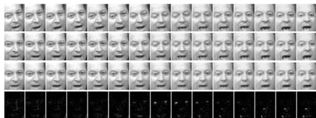
Figure 5. Stabilization of faces in the video. 1st row: frames 1-15 from a 140-frame video, aligned by applying a face detector to each frame; 2nd row: RASL alignment result D \circ \tau ; 3rd row: recovered images A of rank 64; 4th row: sparse error E .
