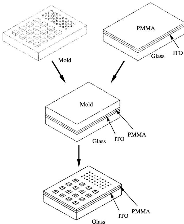
FIG. 1. Schematics of fabricating an OPLED pixel template in PMMA by imprinting.
