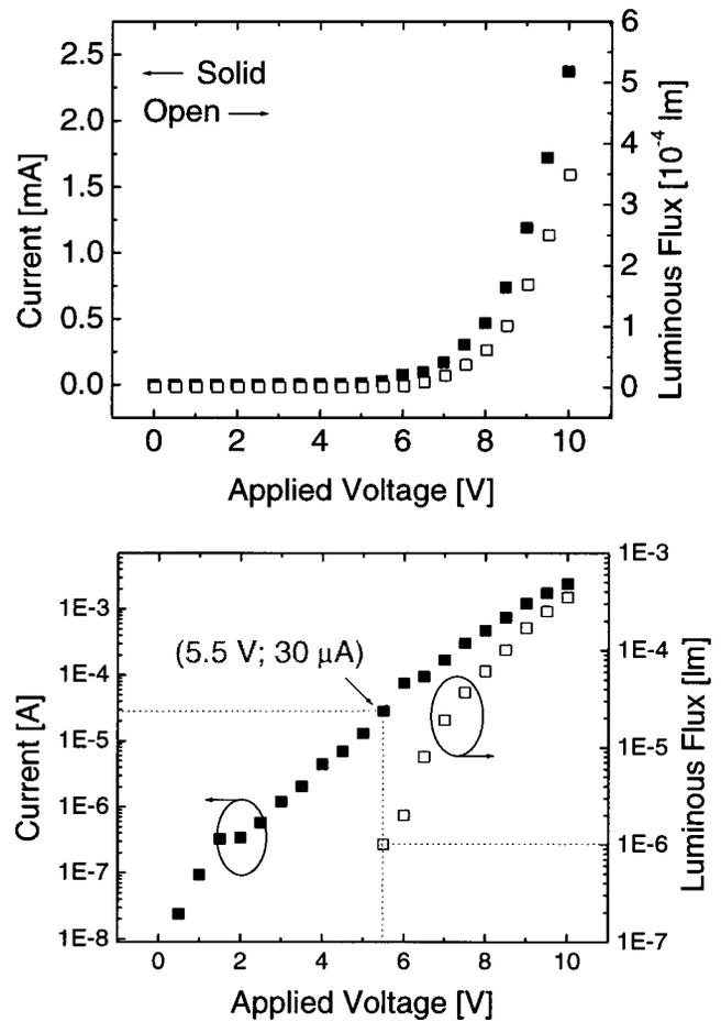
FIG. 5. Current and luminous flux vs applied voltage characteristics of pixel arrays of OPLEDs with ITO/PEDOT/red-emissive polymer/Al structure. The total pixel area is estimated to be 5  $\text{mm}^2$ .
