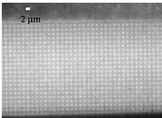
FIG. 4. Optical micrograph of light emission from the smallest size (2  $\mu\text{m}$ ) pixel arrays.
