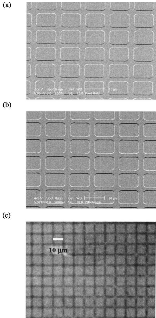
FIG. 2. Scanning electron micrographs of (a) pixel patterns on the mold and (b) imprinted pixel template in PMMA, and (c) optical micrograph of lighted OPLED arrays taken by a charge coupled device camera mounted on a microscope. The pixel size is  $10 \mu\text{m}$ , and the light emission from the pixels is red.
