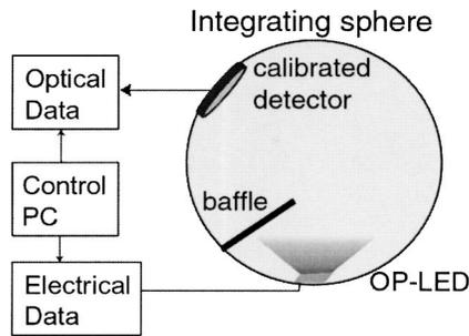
FIG. 3. Schematics of the optoelectronic property characterization system.
