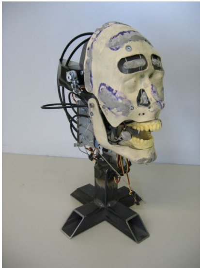
Fig. 5. Mechanical construction of the humanoid robot head
