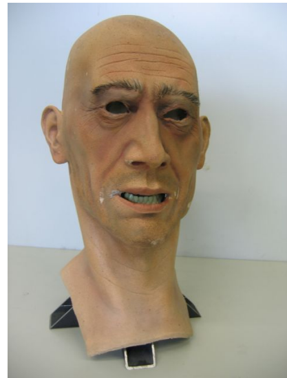
Fig. 4. Mechanical design of the humanoid robot head with the silicon skin. The silicon mask is designed by the company Clostermann Design Ettlingen,Germany
