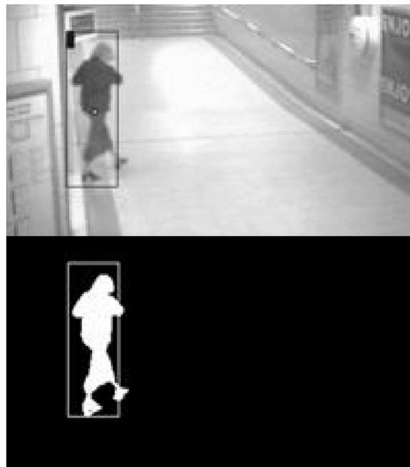
**Fig. 3** Example of background subtraction technique used in motion detection. In this example a bounding box is drawn to fit the object detected
