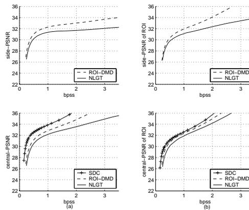
**Figure 1.** Central and side PSNR vs. bits per source symbol (bps); (a): the whole image; (b): ROI subimage
