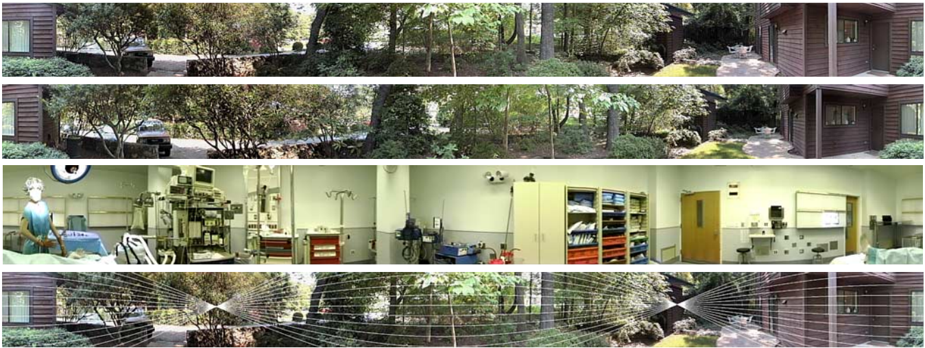
FIGURE 5. Cylindrical images a and b are panoramic views separated by approximately 60 inches. Image c is a panoramic view of an operating room. In image d, several epipolar curves are superimposed onto cylindrical image a.
