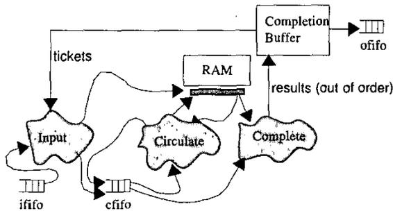
Figure 7. Circular pipeline architecture.
