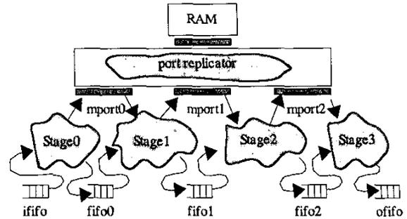
Figure 6. Flexible pipeline architecture.
