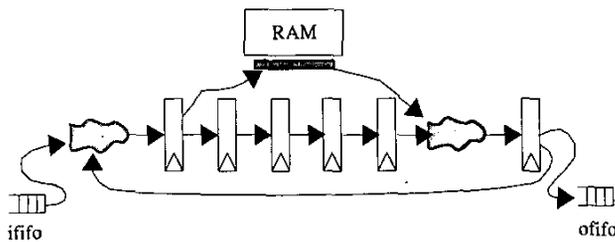
Figure 5. Rigid pipeline architecture
