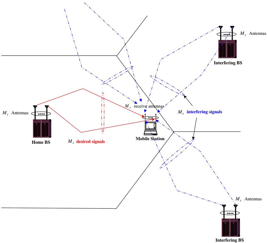
Fig. 1. Other-cell interference in MIMO cellular systems
