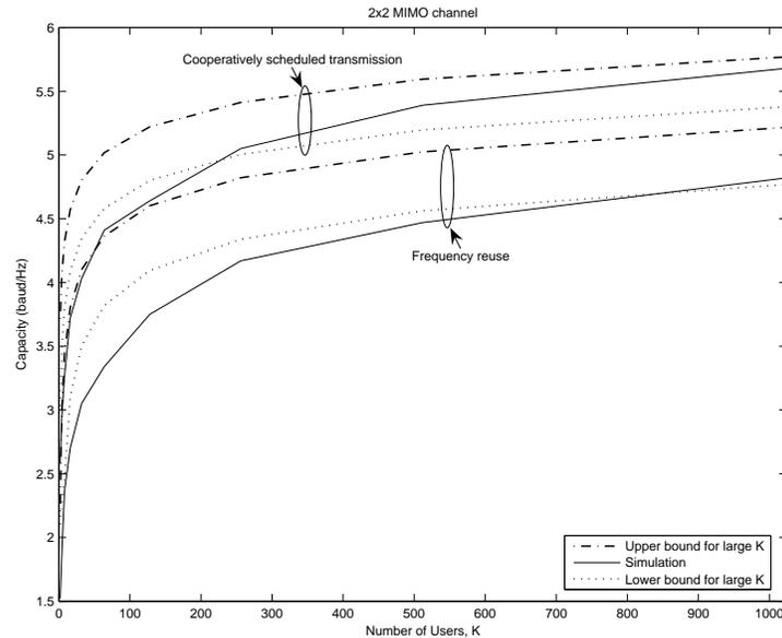
Fig. 4. Shannon capacity of TDMA systems with cooperatively scheduled transmission and with dynamic frequency reuse ( $f = 7$ ). The expanded multiuser diversity gain from cooperatively scheduled transmission is about 1 bps/Hz.
