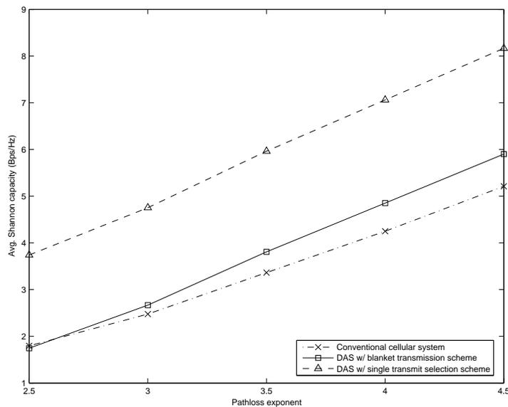
Fig. 6. Average ergodic capacity with CSIR versus the pathloss exponent for one transmit and receive antenna. The capacity gain from distributed antenna systems is dramatic even with universal frequency reuse.
