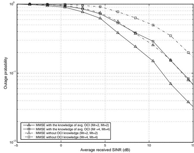
Fig. 3. Outage probability of a cellular MIMO system with target  $E_b/N_0 = 1.5\text{dB}$ . The shadowing is assumed to have  $\sigma = 8\text{dB}$  for interference and  $2\text{dB}$  for the desired user. Note that even with this very low target  $E_b/N_0$ , the outage probability is very high.
