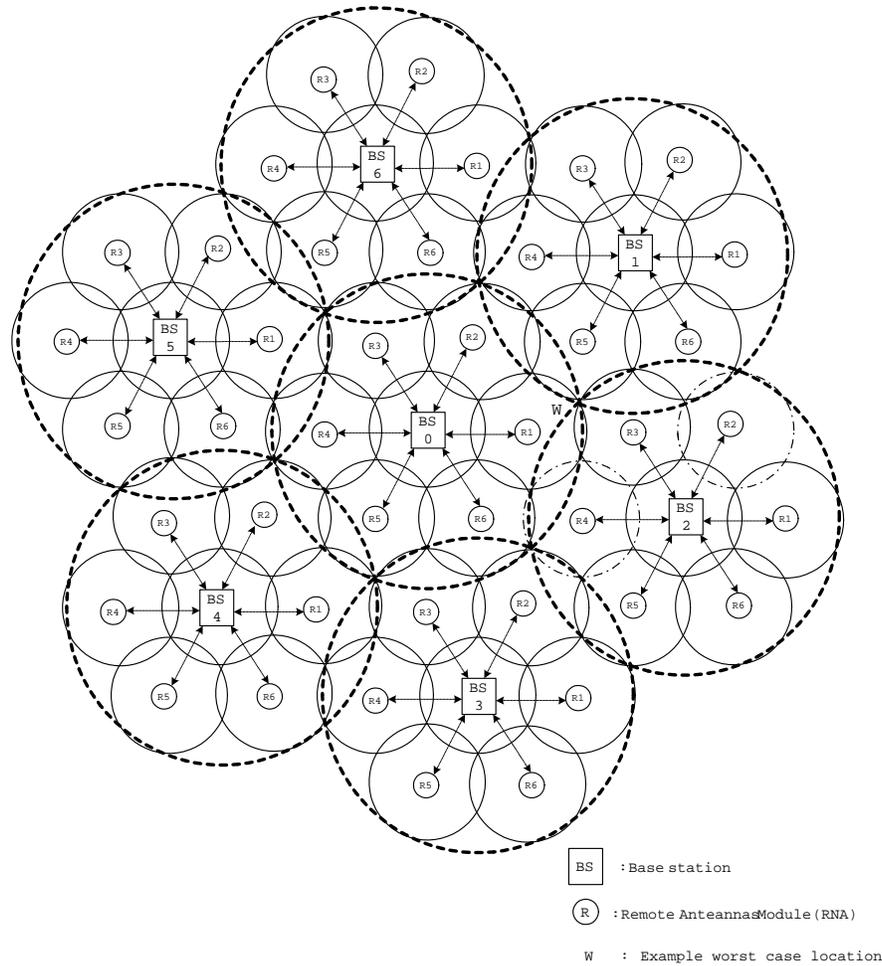
Fig. 5. An example of a distributed antenna cellular architecture for 7 cells, each serviced by 7 total antennas – one at the original base station and 6 remote antenna modules that are spread throughout the cell.
