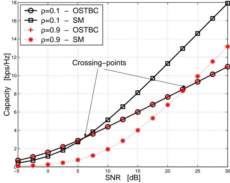
Fig. 2. Capacity of spatial multiplexing and OSTBCs vs. SINR for  $2 \times 2$  MIMO systems with spatial correlation of  $\rho = \{0.1, 0.9\}$  [11].
