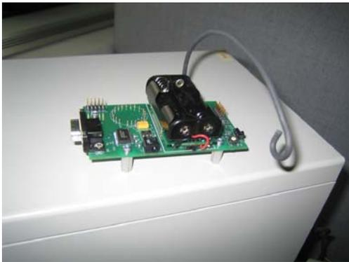
Fig. 2. Picture of MIB510 gateway which uses a serial port with base board attached.
