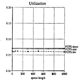
Figure 2: Comparing FCFS utilization derived from theoretical analysis (FCFS-theor), hardware measurements (FCFS-hw), and simulation (FCFS-sim).
