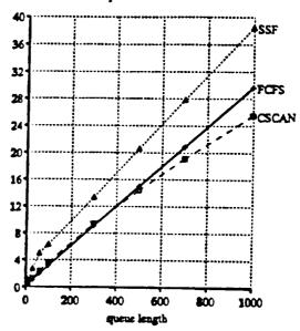
Figure 5: Maximum Observed Response Time for FCFS, SSF, and CSCAN. SSF has significantly worse maximum response time than FCFS, but CSCAN has roughly the same, or lower, maximum response time than FCFS. In some instances, CSCAN is able to have lower response time than FCFS because its average response time is lower.
