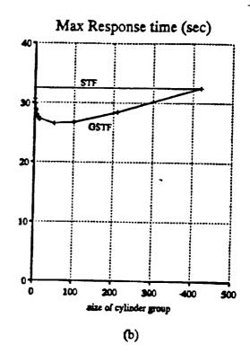
Figure 8: Utilization and Maximum Response Time of Shortest Seek First and Grouped Shortest Time First. Graphed above are the utilization and maximum response times as a function of the cylinder group size. The above results are for queue lengths of 1000.
