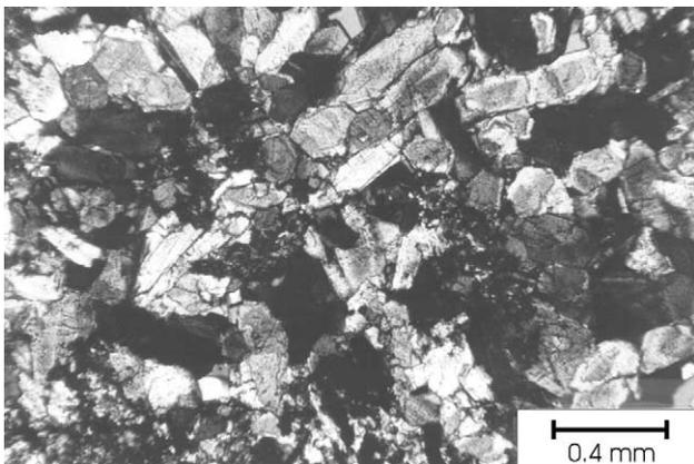
Fig. 4. Thin section of Egyptian Imperial Porphyry with crystals of zoned piemontite.
