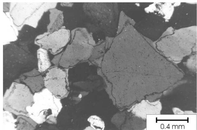
Fig. 11. Thin section of quartzite from Gebel Tingar, west of Aswan. The interstitial space became filled by coaxial crystal overgrowth on the Cretaceous sand grains, caused by precipitation of ascending, silica saturated pore waters towards the Miocene land surface. Crossed polarizing filters.
