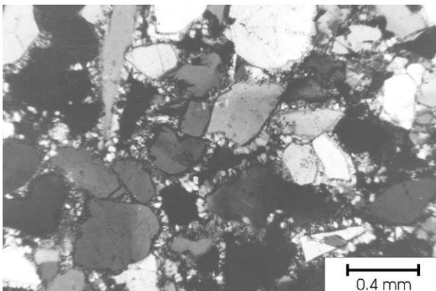
Fig. 10. Thin section of quartzite (silicified sandstone) from Gebel Ahmar near Cairo. Due to a basalt-intrusion the interstitial space of the Oligocene sand grains is filled up with small quartz crystals precipitated from induced hydrothermal fluids. Crossed polarizing filters.
