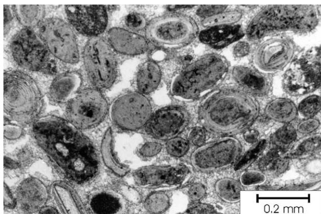
Fig. 13. Thin section of oolitic limestone occurring as ridges parallel to the Mediterranean coast southwest of Alexandria. Crossed polarizing filters.
