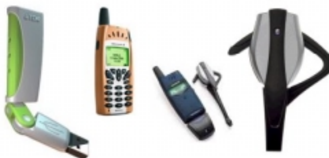
Figure 4 A selection of Bluetooth-enabled products: (from left to right) the TDK USB adapter, the Ericsson R520, Ericsson T28 with Bluetooth module, and the Ericsson wireless headset
