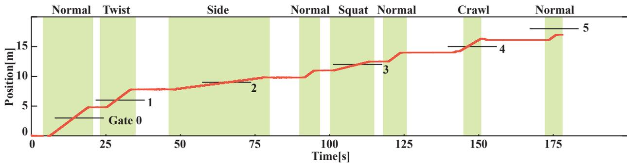
Fig. 9. Simulation result(robot position and locomotion methods)
