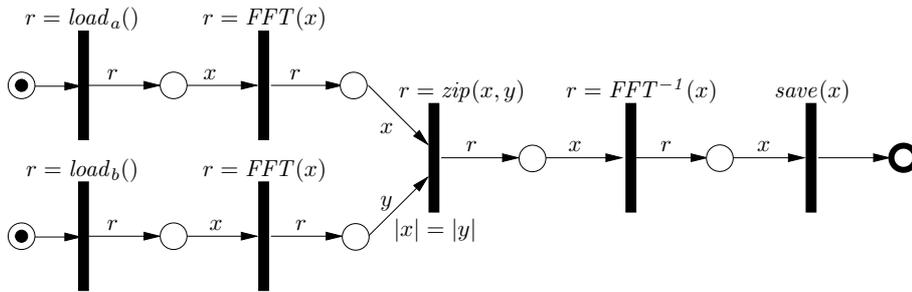
Figure 3: Petri Net representation of convolution program.
