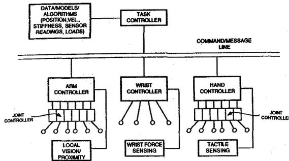
FIGURE 2 SCHEME FOR HAND-WRIST-ARM INTEGRATION
