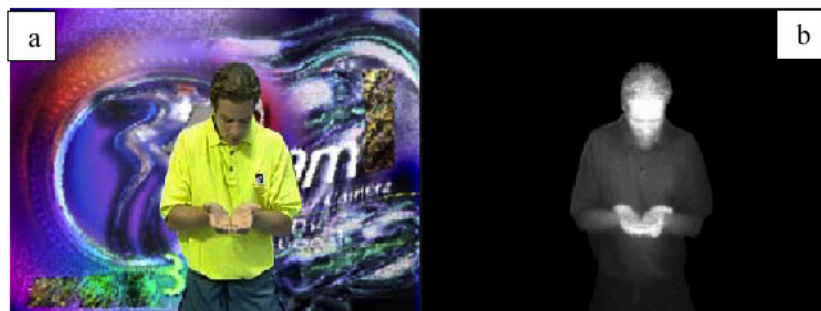
Figure 3: The images taken by the depth camera, a) normal RGB image, b) accompanying depth image: grey level inversely proportional to depth with the [min, max] depth range.
