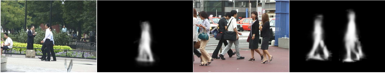
Figure 5. Examples where the flexibility of the Implicit Shape Model leads to overcomplete segmentations. The images show the hypothesized segmentations for some of the pedestrians (only a subset of hypotheses is shown in order to reduce clutter). Since only consistency with a common object center is enforced, superfluous body parts may be assigned to a hypothesis. As a result of this wrong allocation, the scores of neighboring hypotheses may be reduced.
