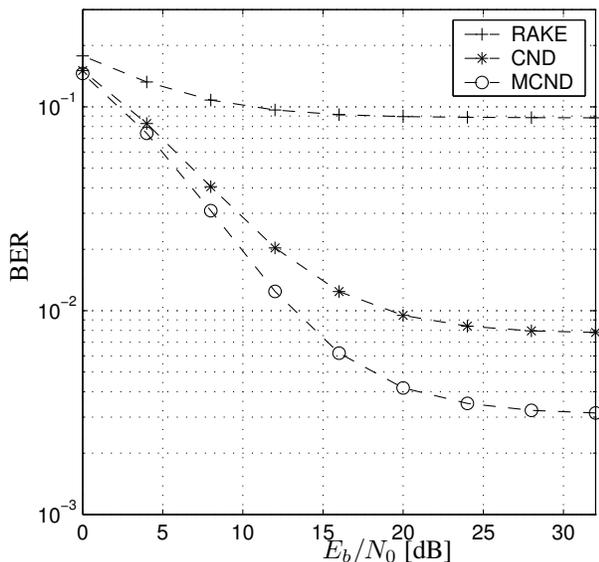
Fig. 1: BER vs.  $E_b/N_0$ . ITU out-to-in B channel.
