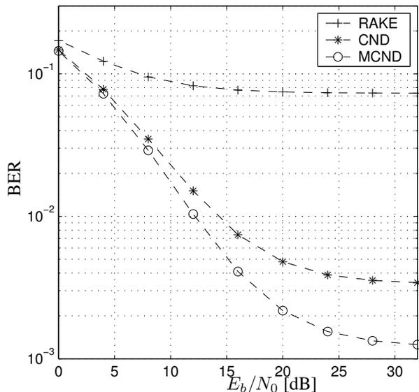
Fig. 2: BER vs.  $E_b/N_0$ . ITU vehicular A channel.
