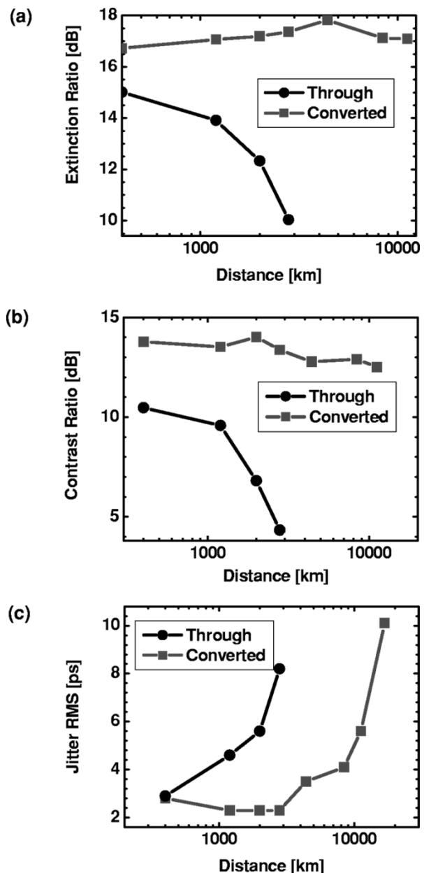
Fig. 7. (a) Extinction ratio. (b) Contrast ratio. (c) Peak-to-peak timing-jitter evolution of the through and converted channel with distance.
