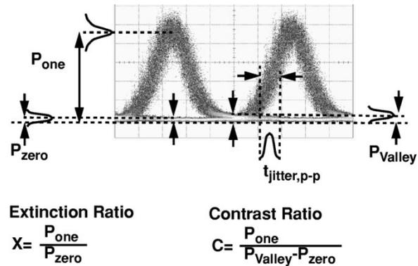
Fig. 6. Eye diagram of the converted channel after 8400 km and definition of extinction ratio, contrast ratio, and peak-to-peak timing jitter as used later.
