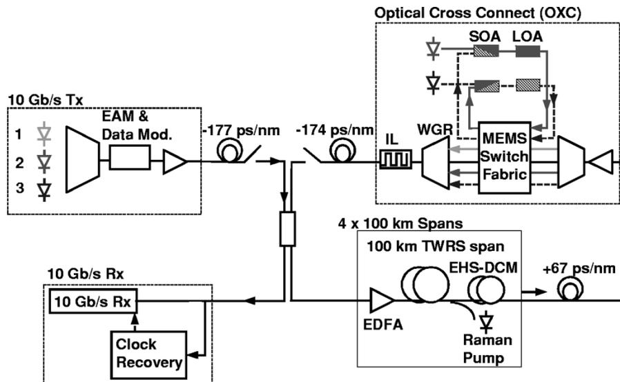
Fig. 3. Loop setup and cross connect to mimic a transparent meshed network.
