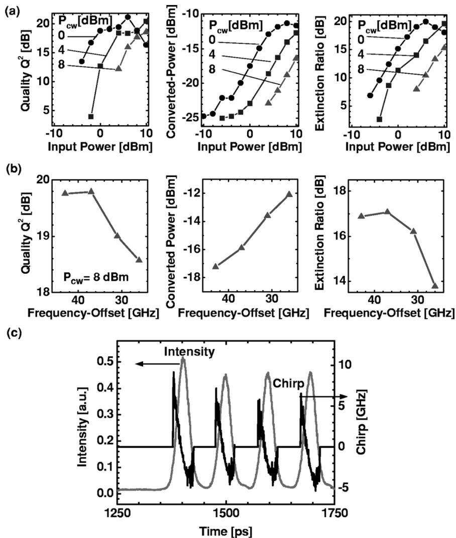
Fig. 2. Wavelength conversion characteristics of the filter scheme at 10 Gb/s as obtained from a single SOA. (a) Dependence of signal quality  $Q^2$ , conversion efficiency and extinction ratio on input signal power and for  $P_{CW}$  laser powers of 0, 4 and 8 dBm. (b) Tolerance of RSOF scheme toward detuning of input-signal wavelength with respect to the edge of the interleaver. (c) Intensity and chirp characteristic of wavelength converted pulse.
