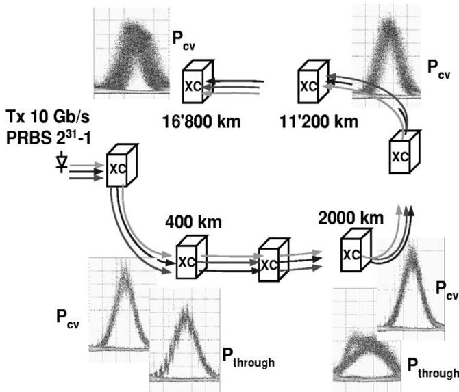
Fig. 5. Eye diagrams of the through  $P_{\text{through}}$  and converted channel  $P_{\text{cv}}$  after 400, 2000, and the converted channel after 11 200 and 16 800 km.
