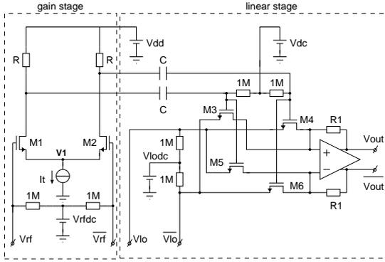
Fig. 4. Mixer with MOS transistors in the linear region
