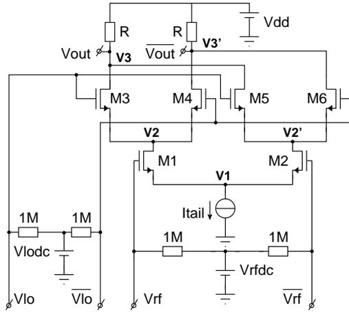
Fig. 2. Double balanced switching mixer
