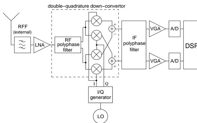
Fig. 1. The double-quadrature low-IF architecture
