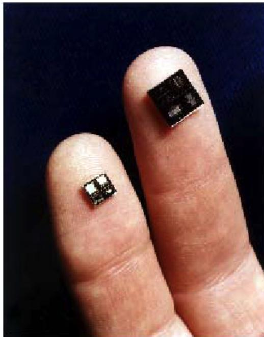
Figure 2: A high performance IMU chip set - accelerometer (left) and gyroscope (right) (from *draperlabs paper*)
