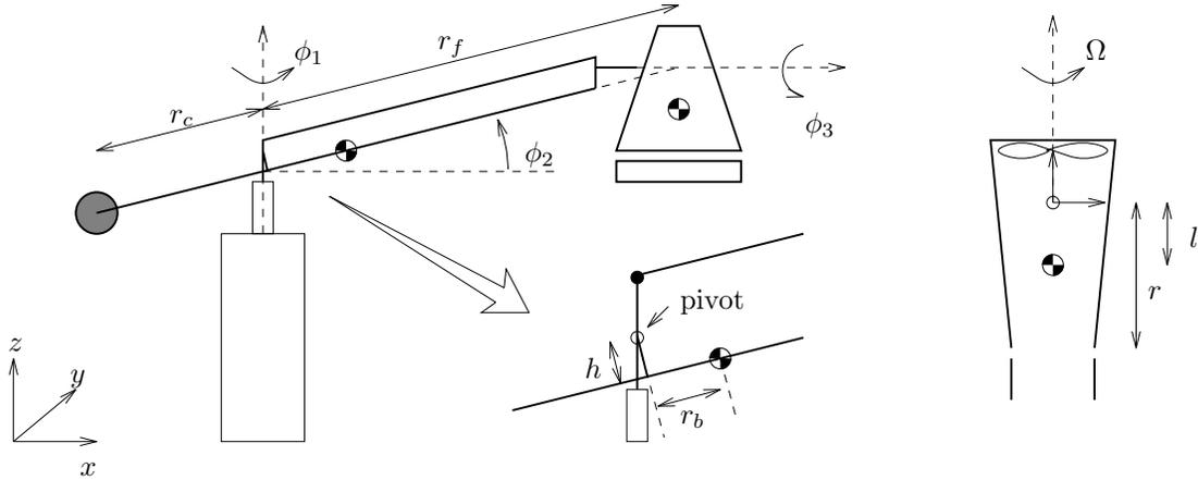
Figure 3: Ducted fan with simplified model of stand.
