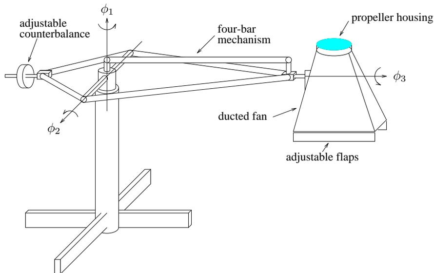
Figure 1: Caltech ducted fan with support stand.
