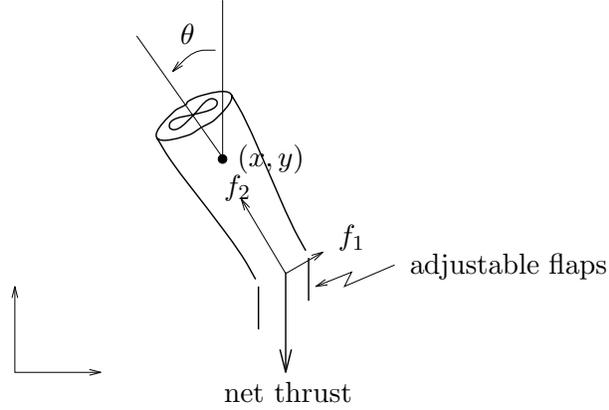
Figure 2: Planar ducted fan model.
