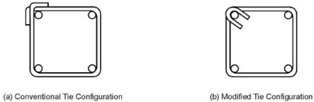
Fig. 4 Conventional and Modified Tie Configuration for Reinforced Concrete Column
