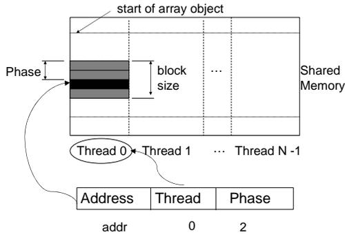
Figure 3. Pointer-to-shared components.
