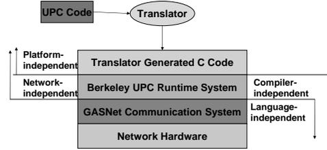
Figure 4. Architecture of the Berkeley UPC Compiler
