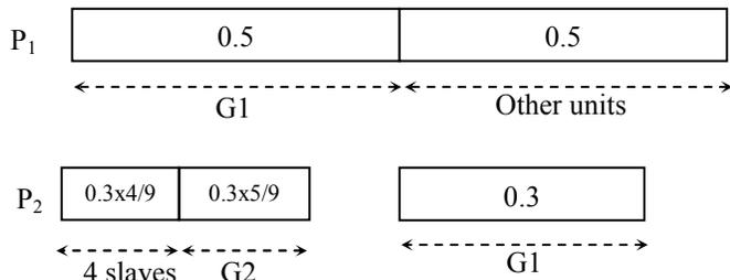
Fig. 4. Polling cycles of masters of P<sub>1</sub> and P<sub>2</sub>
