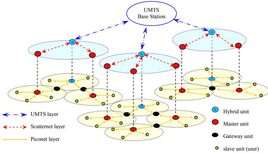
Fig. 1. "Centralized Wireless LAN Architecture" (CWLAN) using Bluetooth and UMTS
