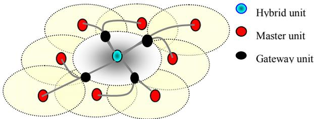
Fig. 2. An example topology of the architecture showing a 3x3 Bluetooth scatternet
