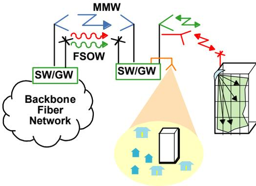
Fig. 1. All wireless hybrid FSOW/MMW links.
