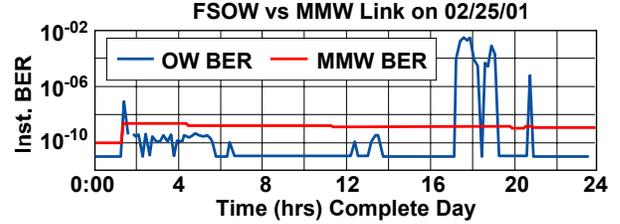
Fig. 2. Hybrid link measure BER
