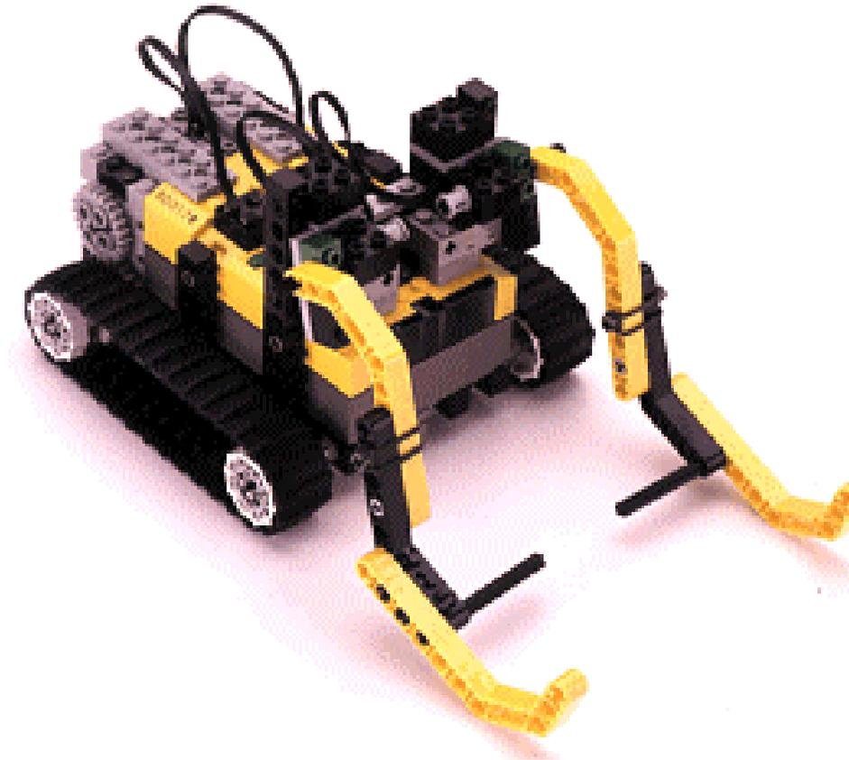
**Figure 1:** The Mindstorms ‘Torbot’ robot body.
