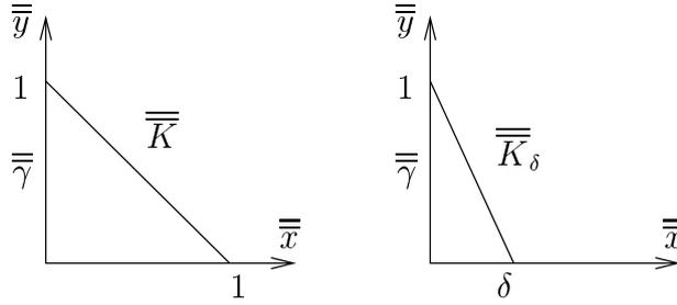
Figure 5: Special face bubble functions definition.
