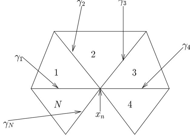
Figure 1: The patch of elements influenced by the basis function  $\theta_n$  .
