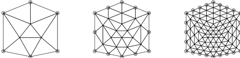
FIG. 1. *Example 1: Nested finite element meshes for MG.*
