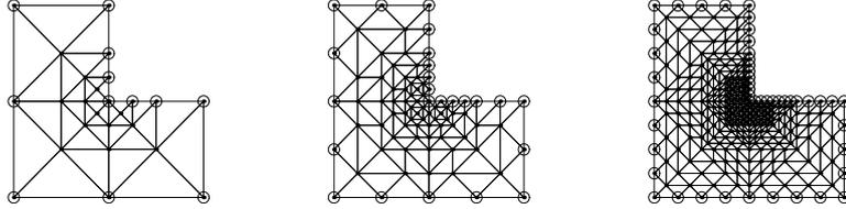
FIG. 3. *Example 2: Nested finite element meshes for MG.*
