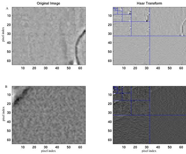
Fig.3 Examples of Haar wavelet transform on sections A (damaged) and B (undamaged). Note spurious lighting effect in top left hand corner of 'clean' image
