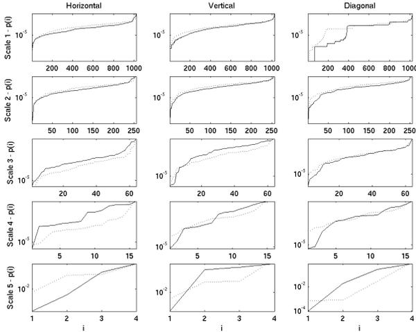
Fig.4 Cumulative normalized wavelet energy distributions for three orientations and five spatial scales. The dotted line represents coefficients associated with the 'clean' image; the solid line corresponds to the 'crack' image (from figure 2).
