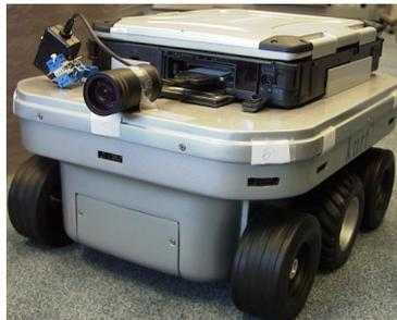
Fig.1 Autonomous KURT2 platform with infrared camera
