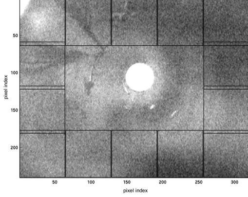
Fig.2 64 \* 64 pixel sections drawn from the periphery of each 320 \* 240 pixel video frame. Note that some overlap was introduced to ensure that the size of the resulting sections were a factor of two
