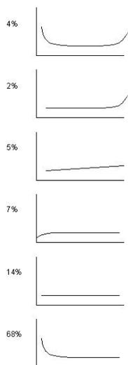
**Figure 3.** The six different conditional-probability curves generated by the United Airlines aircraft study.
