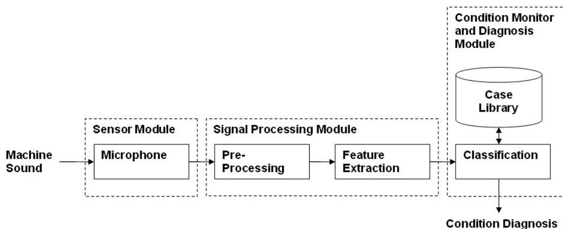
**Figure 5.** Schematic picture of the Case-based fault diagnosis system with its three steps to condition diagnosis.
