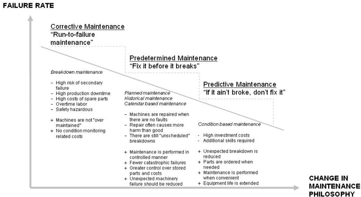
**Figure 2.** Strengths and weaknesses of different maintenance types.
