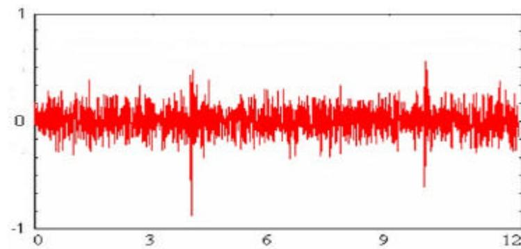
**Figure 6.** Illustration of X+1 recording sample with time/frequency plot from axis 4 on a faulty robot.
