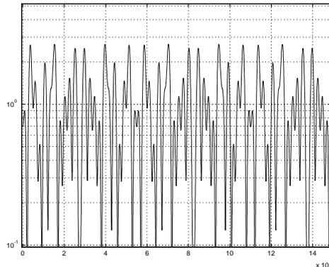
Fig. 5. Spectrum of PAM signal with polarity randomization of the TH sequence. Same positions of the pulses as in Fig. 4, but amplitudes of the pulses given by amp = [-0.5 0.5 0.5 -0.5 1.5].
