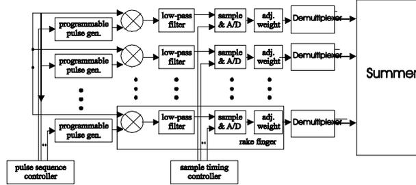
Fig. 6. Structure of Rake receiver for impulse radio.
