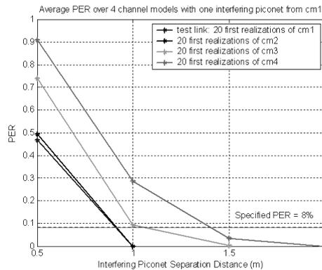
Fig. 12. Packet error rate as a function of the distance of interfering piconet in CM 1.
