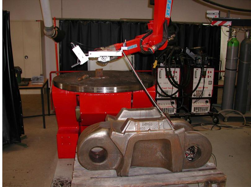
Figure 6: The robot cell with digger chain link, this one is new and unused - to calibrate and test the systems accuracy, the obtained 3D data should fit with the 3D CAD data
