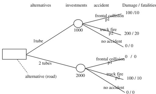
Figure 3. Decision tree for the tunnel example (costs in millions of Euros).
