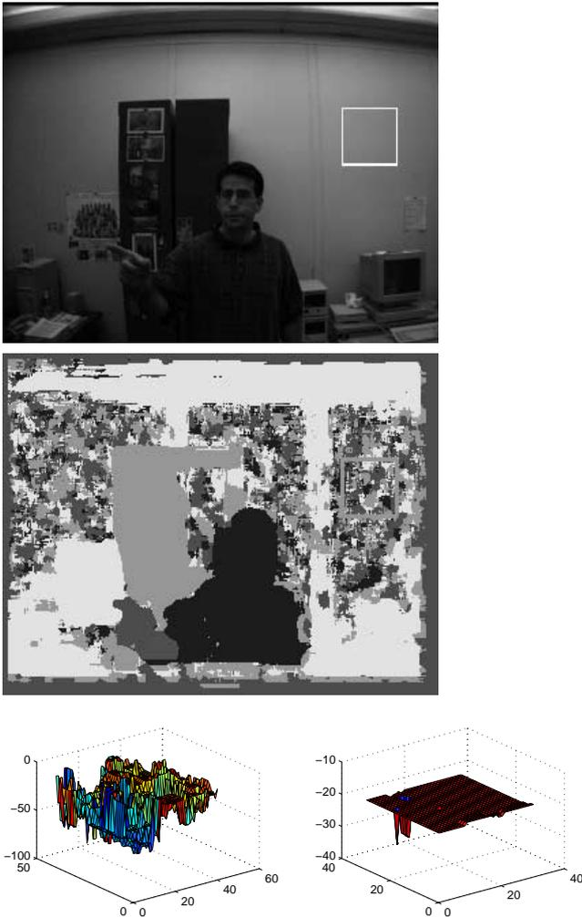
**Fig. 1.** *Top:* Sample input image from camera. *White square* highlights region with little texture. *Middle:* Disparity image from the Digiclops Stereo System from Point Grey Research, Inc. Note noise in the highlighted region. *Bottom left:* Reconstruction of physical surface based on disparity values in highlighted region (negative  $z$  axis trends away from camera). *Bottom right:* Reconstruction of physical surface based on region centered inside of the human figure in the middle
