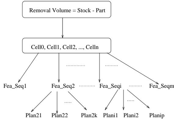
Figure 4. Process Plan Search Space After Expanding Some Feature Sequence Nodes
