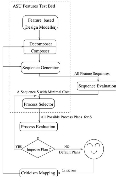
Figure 3. Process Planning System Flowchart
