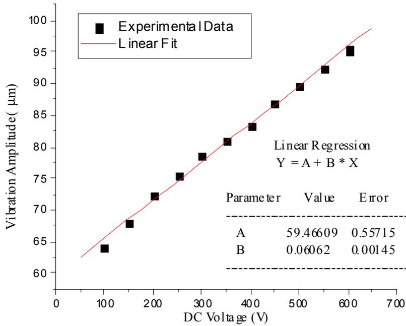
Figure 2: Results of the calibration of the PZT transducer used to calibrate the MR probe. In this case lower voltages were employed.
