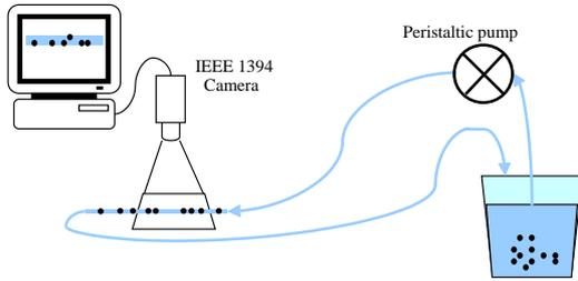
**Fig. 1.** Experimental setup for flow rate measurements.
