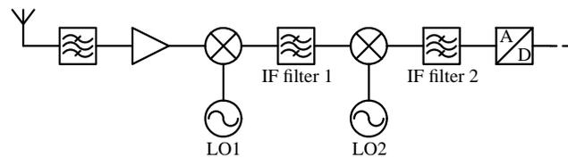
Figure 2: super heterodyne receiver with variable bandwidth IF filter
