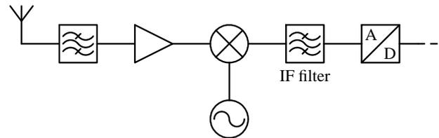
Figure 1: conventional super heterodyne receiver, with fixed bandwidth IF filter
