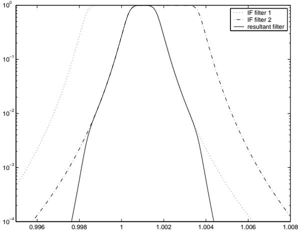
Figure 3: transfer characteristic of two 14<sup>th</sup> order Butterworth band pass filters, one shifted in frequency, and the resultant filter
