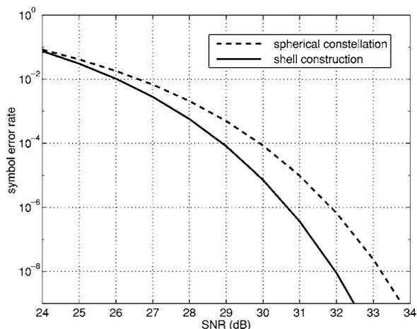
Figure 4. Probability of error for the two shell design and a one shell design of the same cardinality.
