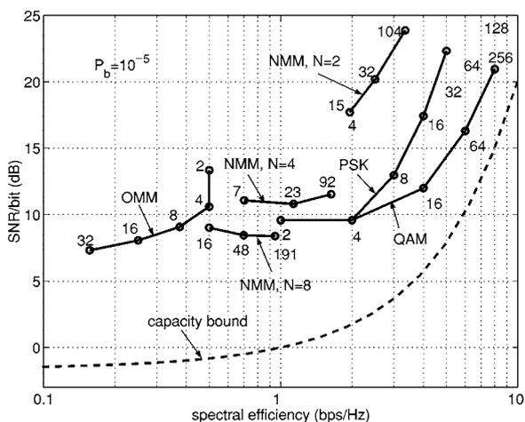
Figure 3. Energy and spectral efficiencies of the noncoherent designs.
