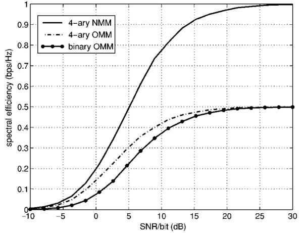
Figure 9. Spectral Efficiencies for noncoherent, coded, OMM and NMM versus the channel SNR per bit for the Rayleigh fading channel. The NMM signals were constructed in a two dimensional basis.
