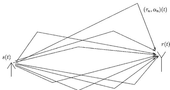
Figure 8. The fading multipath channel.
