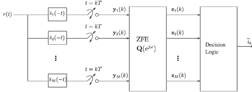
Figure 11. Matched filter receiver front end and ZFE detector.
