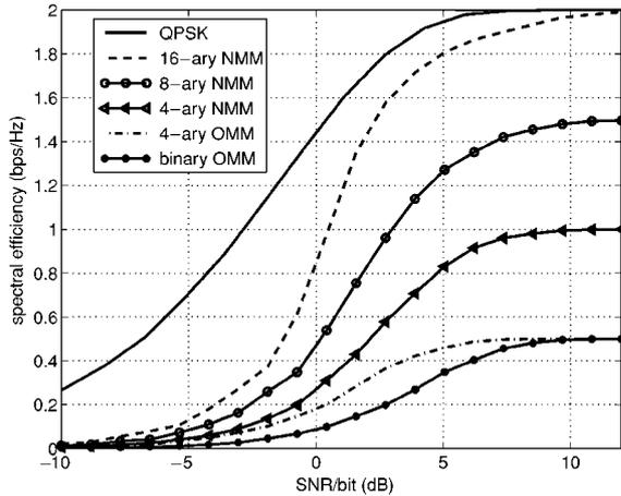
Figure 5. Spectral efficiencies for noncoherent, coded, OMM and NMM versus the channel SNR per bit on the AWGN channel. In each case the NMM signals were constructed in a two dimensional basis. The spectral efficiency of coherent QPSK as derived in [23] is plotted for comparison.
