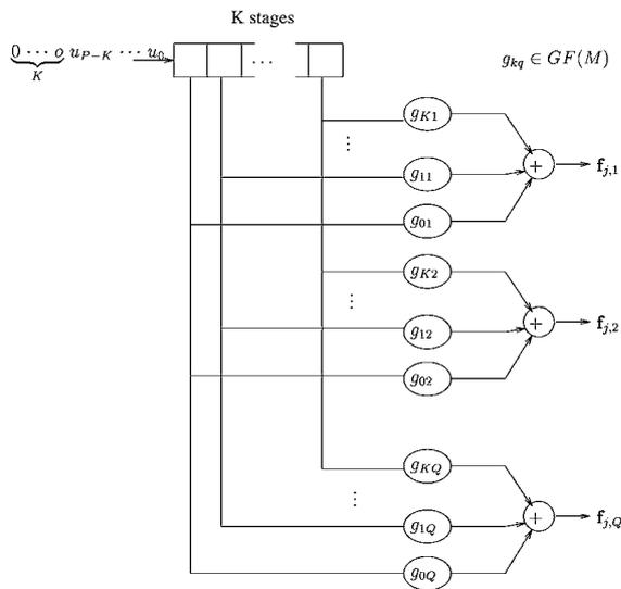
Figure 6. Block diagram of the convolutional encoder.
