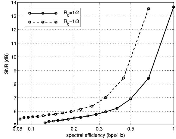
Figure 7. Energy and spectral efficiencies of the noncoherent designs on the AWGN channel with coding on a 16-ary alphabet.
