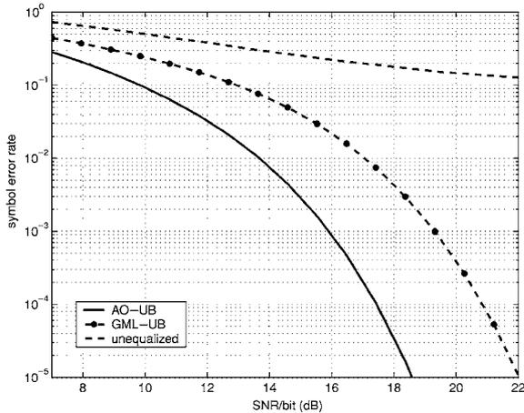
Figure 12. Probability of error for 4-ary FSK over the ISI channel of Eq. (93).
