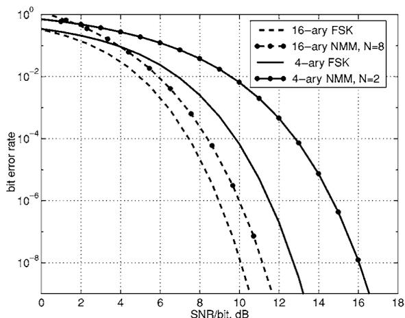
Figure 2. Bit error rate versus SNR for several equal-energy OMM and NMM designs.
