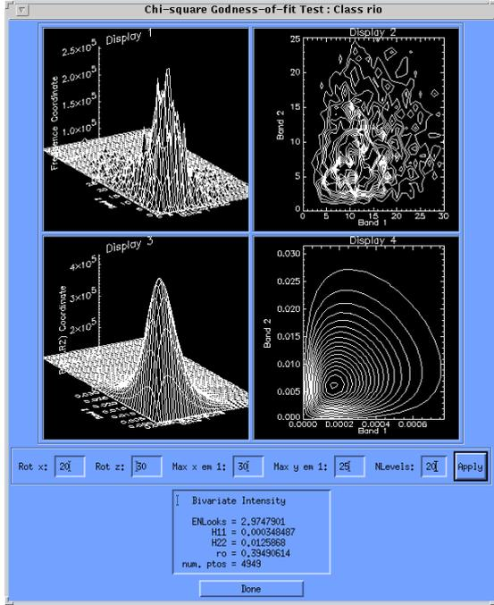
Figure 1 - Density, 2-D histogram, contour plot and estimated parameters of two multilook intensity bands.
