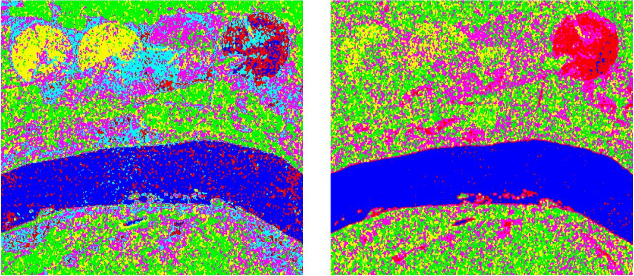
Figure 6 - ML classifications of the L (left, using HV and VV components) and C (right, using HH and HV components) data sets.
