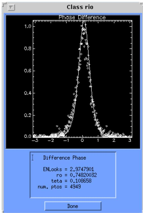
Figure 3 - Histogram, fitted density and estimated phase difference parameters.
