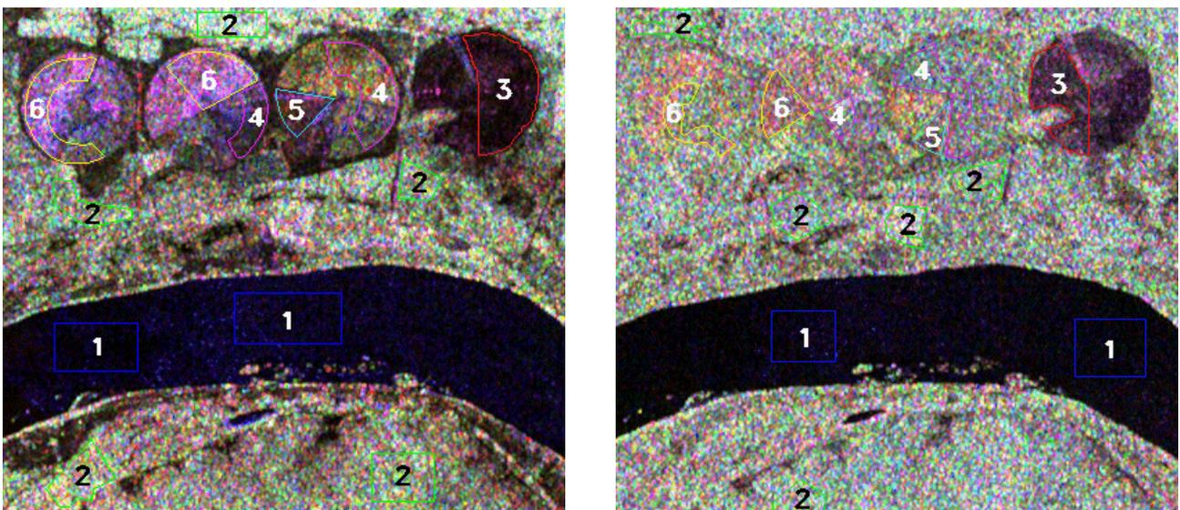
Figure 5 - Two colour compositions of the original data R-HH, G-HV, B-VV, bands L (l) with training sets and C (r) with test sets.
