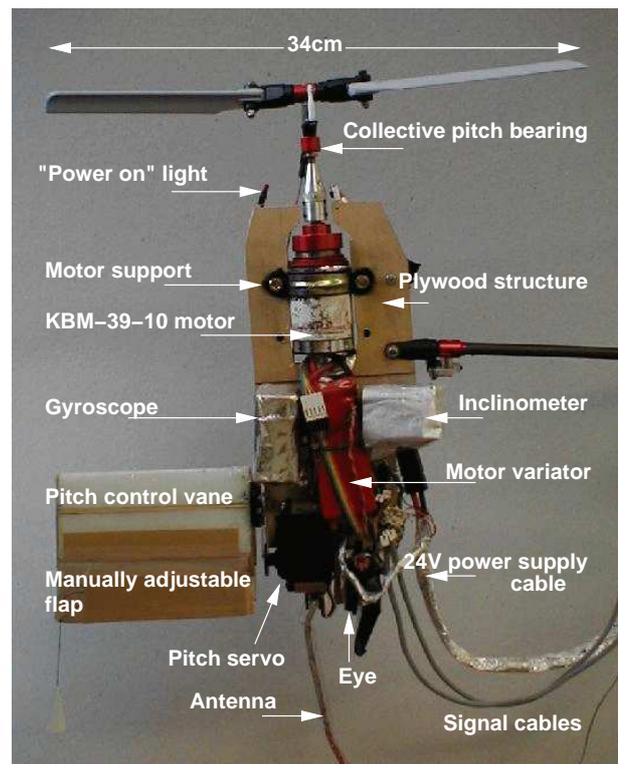
**Figure 6:** The visually-guided *Fania* rotorcraft weighs 0.84 kg (front view).
