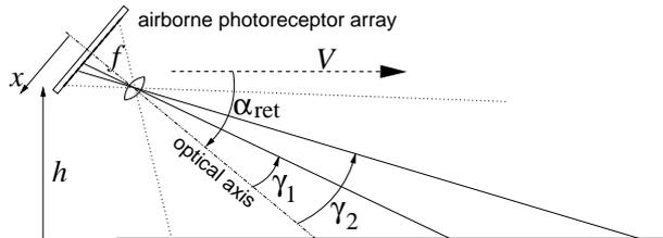
**Figure 2:** Airborne eye with single lens and linear photoreceptor array moving at altitude  $h$  and horizontal speed  $V$  above ground.
