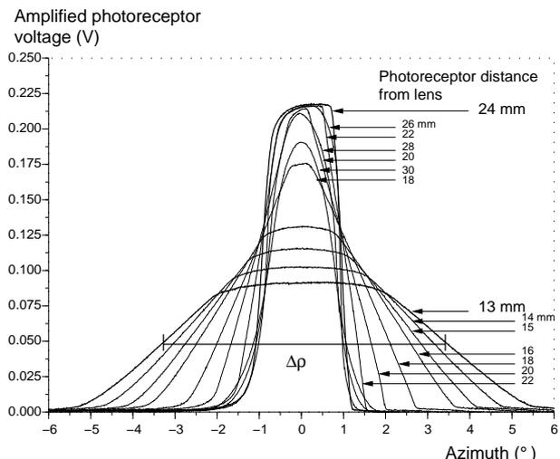
**Figure 3:** The Angular Sensitivity Function (ASF) of a single photoreceptor (width 0.8mm) behind the eye lens is projected onto the photoreceptor array for 11 defocusing distances ranging from 13 to 30mm.
