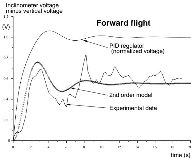
**Figure 7:** Experimental data fitted with a second-order model of the pitch response to a 60% step deflection ( $+28^\circ$ ) of the elevator vane for forward flight. Experimental data is digitized at 20 Hz and smoothed over 5 samples. The top curve plots the normalized pitch response to a step input following PID tuning (sample rate = 20 Hz) of the second-order model.
