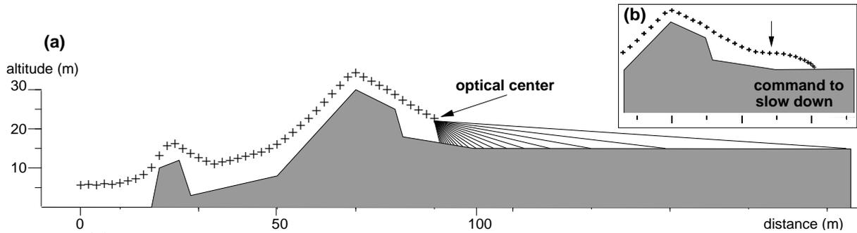
**Figure 5:** (a) Simulation of terrain following with the 20-photoreceptor retina's optical axis set  $-40^\circ$ . The FOV is  $75^\circ$  in the vertical plane, i.e., within the lens's physical limits.  $V = 2$  m/s,  $h_{init} = 5$  m, iteration step = 1 s. (b) An automatic landing was simulated by linearly decreasing the aircraft horizontal speed by 10% of the initial reference speed at every iteration while retaining the same request to maintain a reference OF condition.
