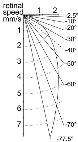
**Figure 4:** Polar plot of equation (1) : retinal speed (mm/s) vs ray angle (deg) around the optical axis of the retina ( $\alpha_{\text{ret}} = -40^\circ$ ,  $f = 13$  mm,  $V = 2$  m/s,  $h = 5$  m).
