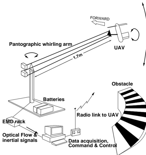
Figure 1: Whirling-arm test bed.
