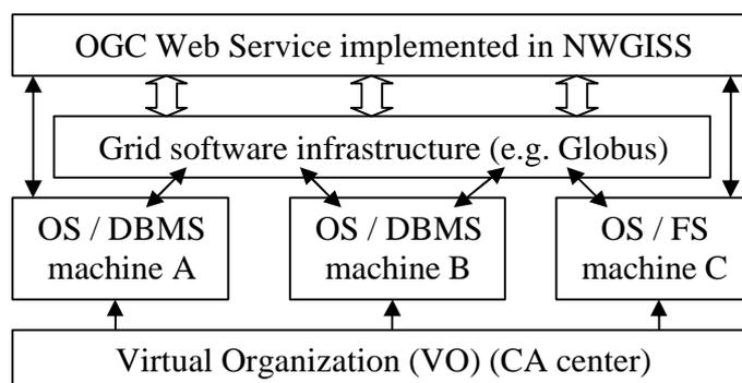
Fig. 1 Integrating Grid technology with OWS I
