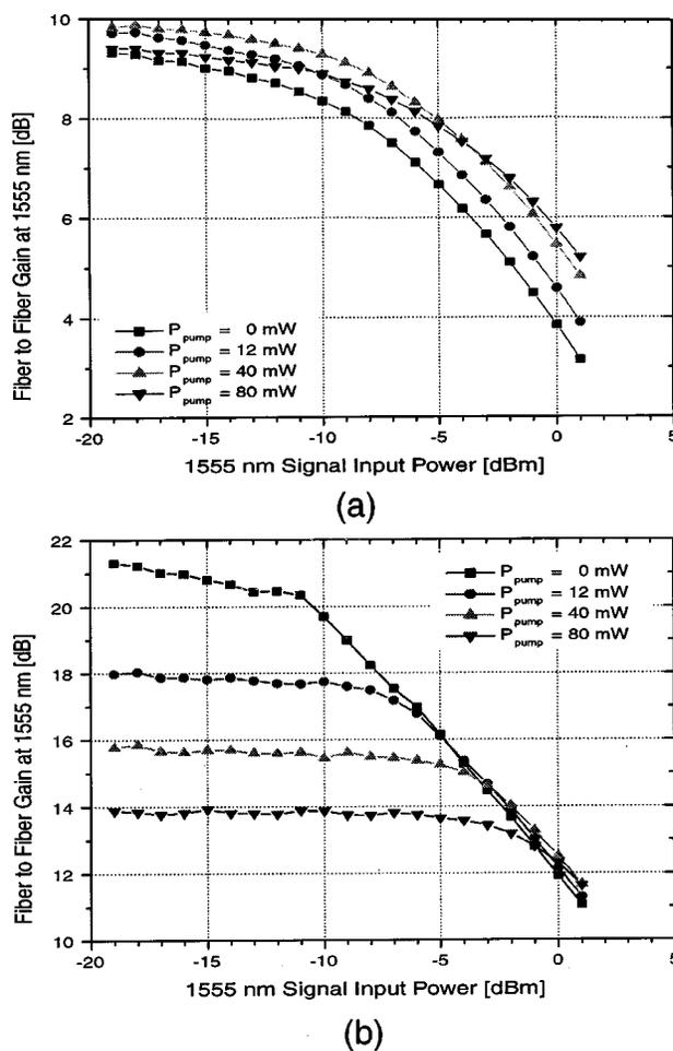
Fig. 2. Saturation behavior of the SOA for different injected 1480-nm pump powers. (a) SOA current is 150 mA. (b) SOA current is 450 mA.
