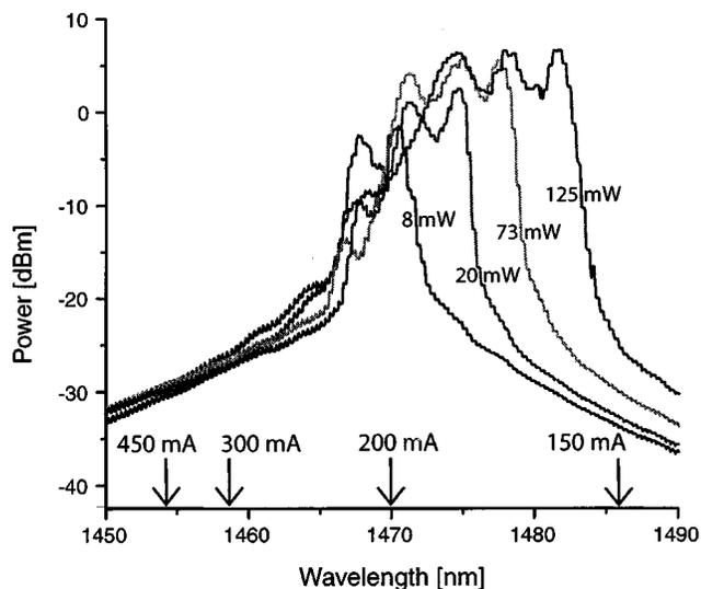
Fig. 1. Pump output power spectrum for different output powers. On the x axis the material transparency wavelengths are indicated for four different SOA bias currents.
