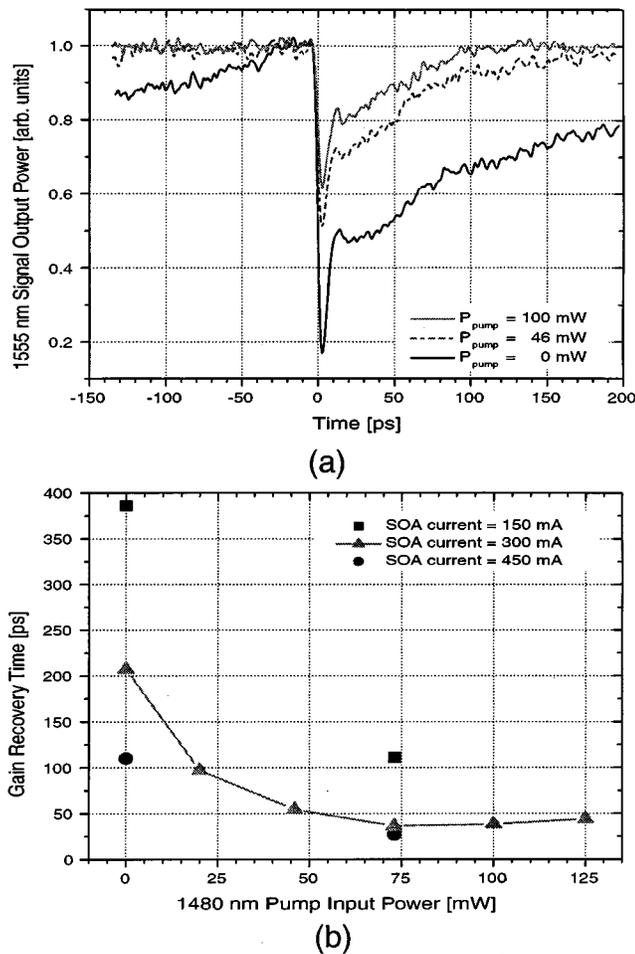
Fig. 4. (a) Streak camera measurement of the gain recovery for a SOA current of 300 mA with no pump input power and 73 mW of pump power. (b) Extracted exponential gain recovery time as a function of injected pump power for different SOA currents.
