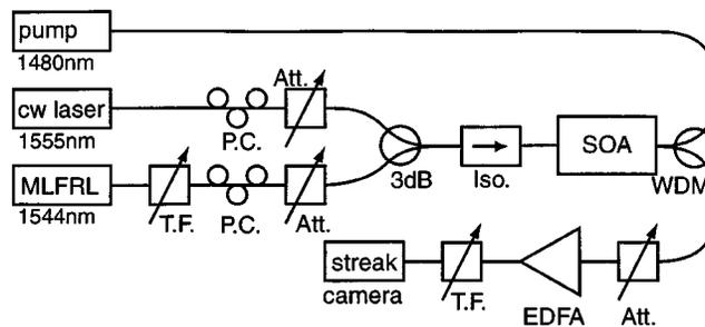
Fig. 3. Experimental setup used for the gain recovery characterization of the SOA with 1480-nm pump injection. MLFRL = mode-locked fiber ring laser. P.C. = polarization controller. T.F. = tunable filter. Att. = attenuator. Iso. = isolator. WDM = 1480/1550 coupler.
