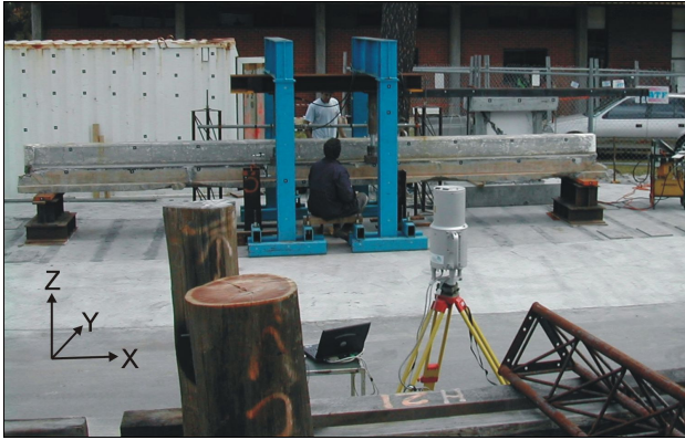
Figure 2. Concrete beam and the Riegl LMS-Z210.
