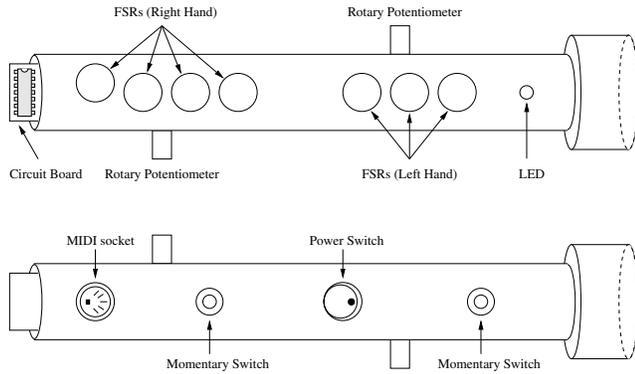
Figure 2: *The Pipe* layout diagram: View from above (top) and below (bottom).
